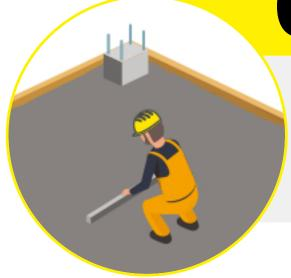
Firstly, get the screeding done. In screeding, the upper layer of the excess concrete is removed.
