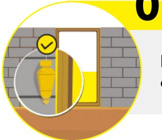
Plum bob is used for correct alignment of the frames.
