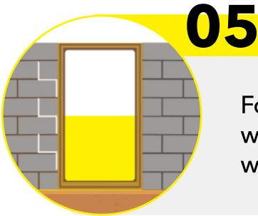
For doors 3 holdfasts are used and two for the windows and afterwards those are filled with the concrete.
