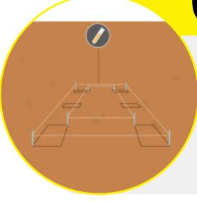
After deciding the pillar placement, mark the area for excavation with the help of a chalk powder; before starting the work of excavation, do not forget to get the soil tested.
