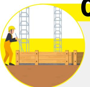
The shuttering position of the beam should be kept solid before pouring the concrete. Give 25 mm cover to the rods in the beam and fill the conrete after properly compacting it.
