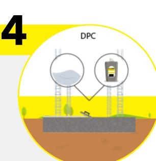
If the plinth beam has not been layed, get the Damp Proof Course (DPC) done on the foundation to make your house waterproof and then start constructing walls. Do not forget to mix waterproofing agent like UltraTech ILW/ILW plus in the DPC.
