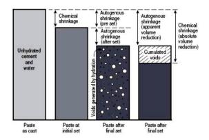
autogenous concerns as the mixtures are using more "special" cements and multiple admixtures while reducing water. It is a problem often associated with high-strength concretes which typically contain high cement content and low water-cement ratio. This shrinkage occurs in the interior of large concrete mass and tends to increase at higher temperature. The magnitude of the shrinkage is found to further increase if silica fume has been used in the concrete mixture.
