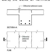
settlement of the solids. These obstructions 'break the back of concrete' and generate voids under their 'belly' as shown. As a result, cracks are formed directly over formwork tie bolts or over the reinforcement near top of a section due to the
