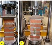
30% increase in masonry strength was observed in mortar made with Manufactured Sand. Stack bonded masonry prism under compression test Fig (a) Typical failure pattern, Fig (b) Prism with strain gauge
