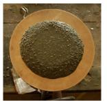
measured by conducting a flow table test as per code guidelines (BS - 4551). 1:6 Mfd. Sand mortar at 85% flow
