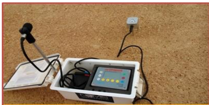
Blast Vibration Monitoring
